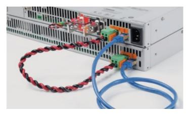
Figure 2. N7909A power dissipater unit rear connections to a 1 kW APS power supply.
