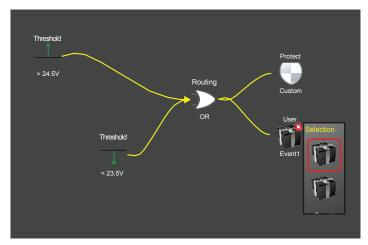
Figure 4. Configuring a trigger expression with the N7906A Power Assistant software.
